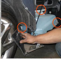
Use the enclosed bracket to move the bottle 1" back and a zip tie to secure it on the top factory hole.
