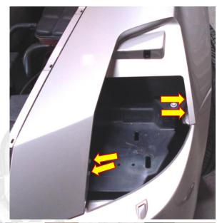
To get to the last bolts/clips you will have to pull back on the weather strip at the bottom of the windshield as shown.
