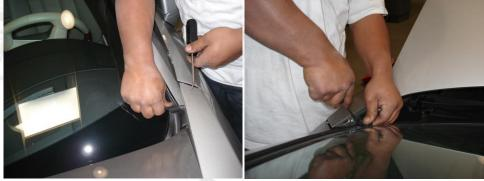
After removing all the bolts and clips from the fender you should be able to remove the fender with the help of your helper.
